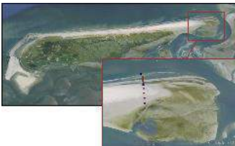
Figure 1: The instrument array on Schiermonnikoog consisted of 3 frames (blue squares) equipped with Acoustic Doppler Velocimeter (ADV)s, pressure sensors and Optical Backscatter Sensors (OBS), and 9 stand-alone pressure sensors (orange squares).
