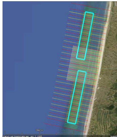
Figure 1: The planned design of the nourishment at Heemskerk. The cyan rectangles show the northern and southern nourishment sections. Red lines show the annual Jarkus transects; Yellow and green lines show the high-density survey lines of the ‘Jarkus verdicht’ surveys and the Shore jetski surveys near the end sections.
