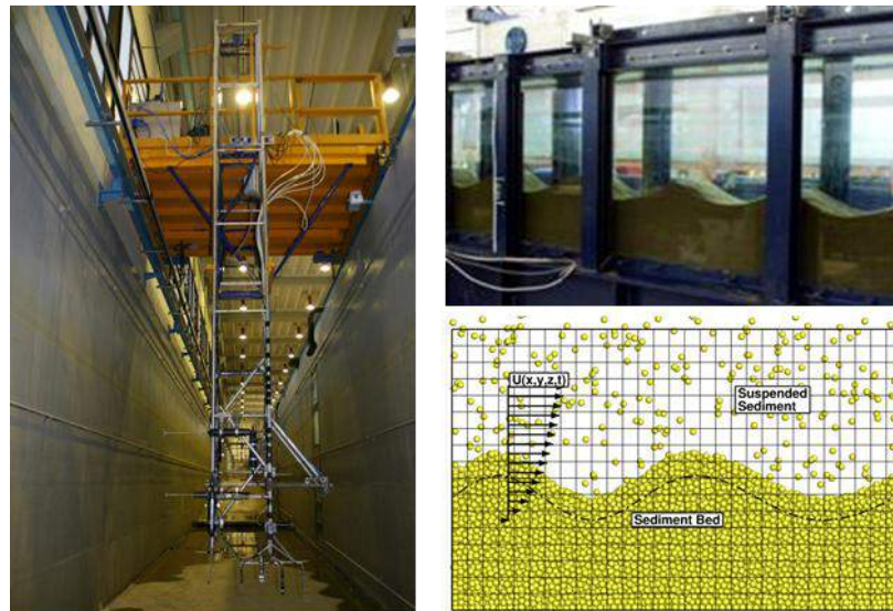
Figure 1. Left: Barcelona wave flume; Upper right: Aberdeen Oscillatory Flow Tunnel; Lower right: illustration two-phase numerical model.
