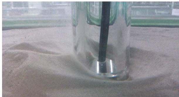
Figure 1. Initiation of scour hole formation during experiment
