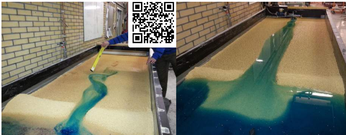
Figure 1. Experimental estuaries without (left) and with river inflow (right). QR: movie of a short tidal basin in large-scale equilibrium with sustained bar and channel dynamics.
