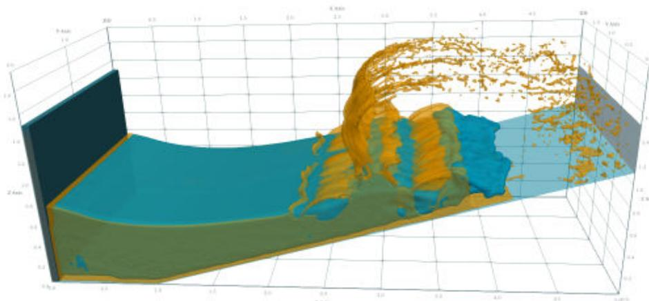
*Three-dimensional interaction of breaking waves and backrush produced by an idealised wave maker. Overlay of the flow at the same instant resolved by SPH with 400k (blue shades) and 27M (yellow shades) elements*
