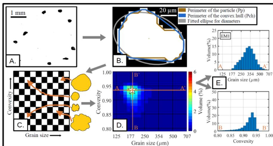
Figure 1 (A) Binary image of sediment grains. (B) Computation of particle characteristics. (C) Assignment of grains to size-shape classes. (D) Grain size-shape distribution (SSD). Star marker designates the mode of the distribution. (E) Grain size (upper panel) and grain shape (lower panel) cross-sections through the SSD along respectively A-A' and B-B'.
