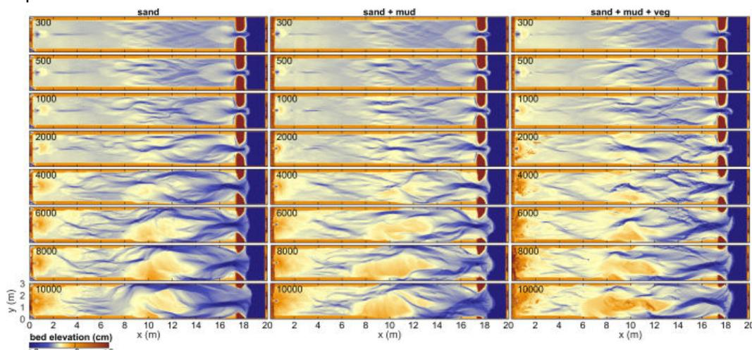
Figure 1 Morphological development of three net infilling estuaries with the number of tidal cycles in the upper left corner for each DEM.
