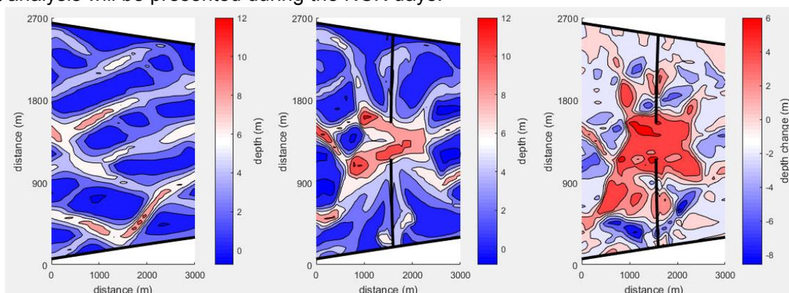
Figure 1 Bathymetry of Delft3D model runs without cross-sectional area reduction (left), and with (middle), and map showing the difference between the two with erosion in red and deposition in blue (right), duration=30 years
