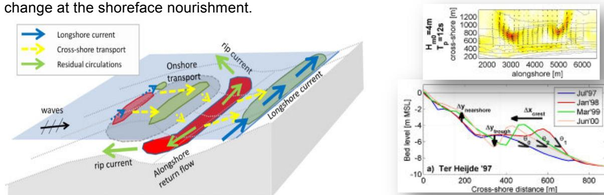
Figure 1 Overview of relevant processes for the redistribution of shoreface nourishments (left panel), an illustration of computed impact of shore-normal storm waves (top-right panel) and an illustration of the measured cross-shore reshaping of a shoreface nourishment at Ter Heijde (lower-right panel).
