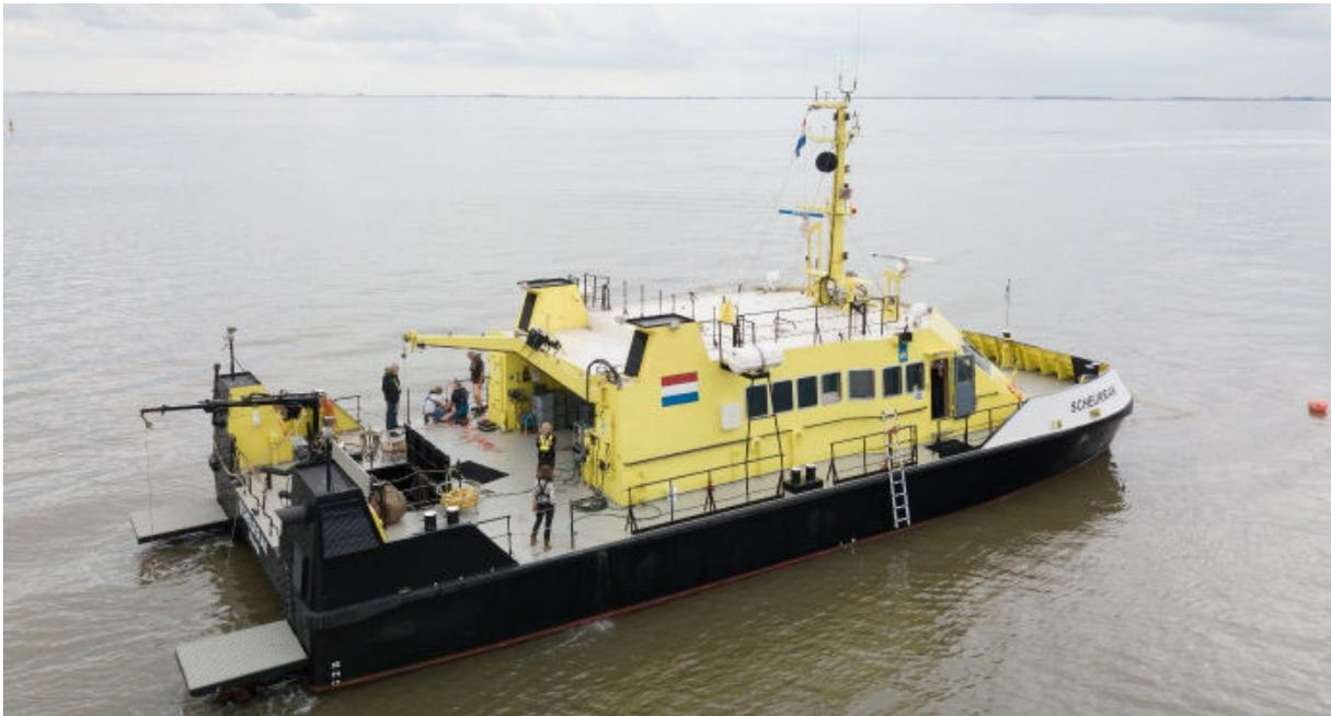
Figure 1 Survey Vessel Scheurrak equipped with ADCP, MBES, SBES, ABS, CTD, OBS, LISST and pump systems.
