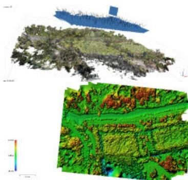
Figure 1 Example of drone imageries processed with SfM photogrammetry. Top: Mangroves dense point cloud. Bottom: SfM
