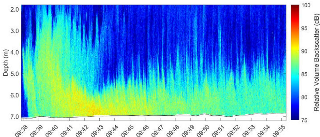
Figure 1 Non-pulse compressed echogram from a vessel-mounted Signature1000 with 5 cm pixels that extend down to the sea bed at a depth of approximately 7 m.
