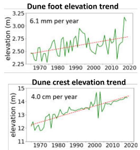
Figure 2 Dune foot and crest elevation through time
