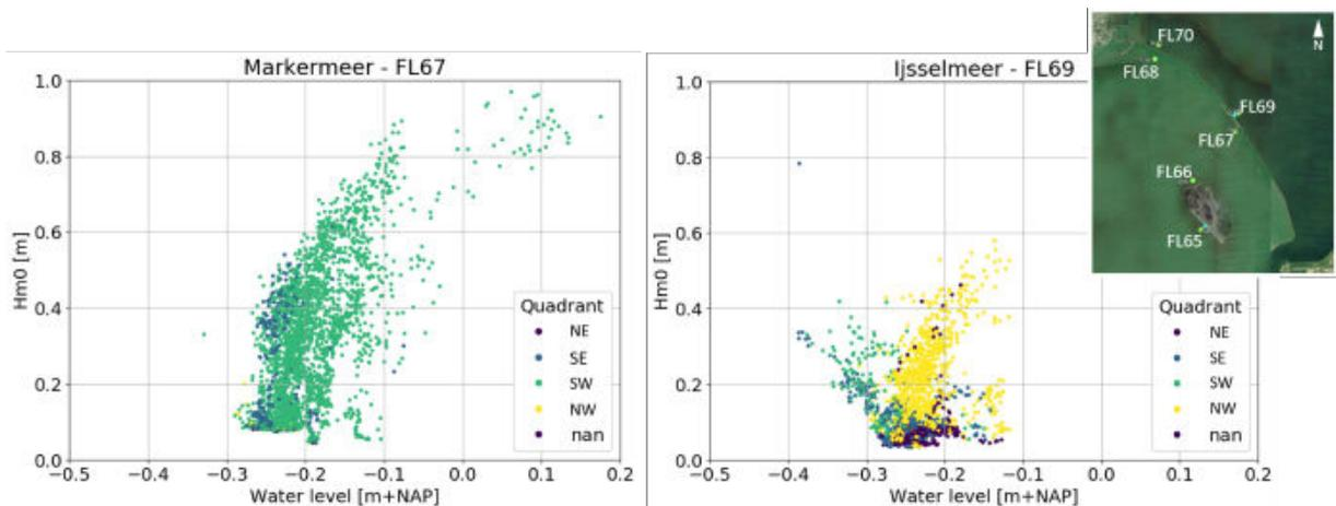
Figure 1 Correlation water level and wave height from ADV measurements
