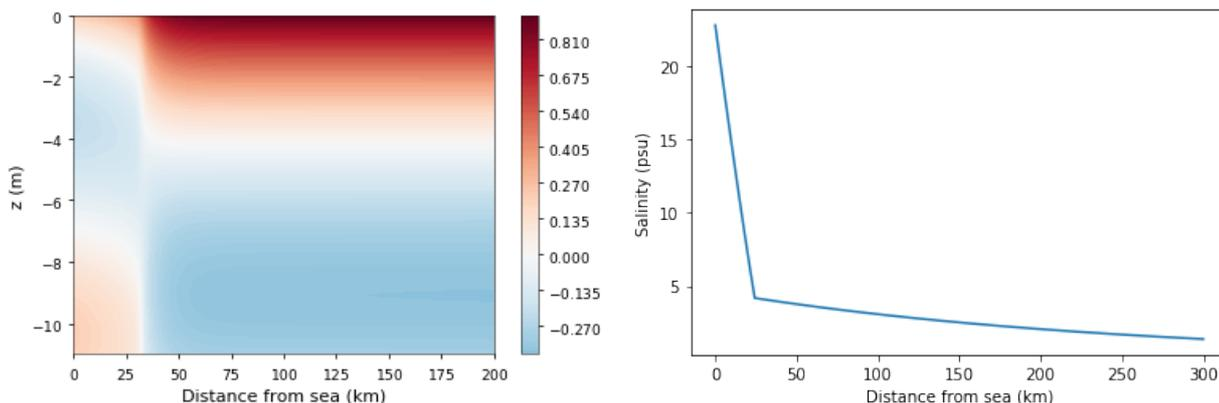
Figure 1 Horizontal water velocity (m/s) (left) and vertically averaged salinity (right) for weak up-stream wind.
