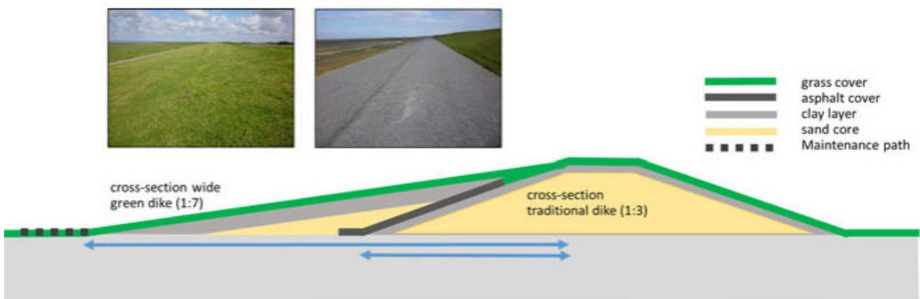
Figure 1 Cross section of a traditional dike and a wide green dike. Source: Van Loon-Steensma and Vellinga (2019)
