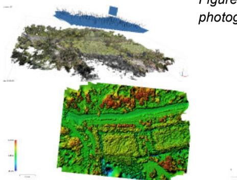
Figure 1 Example of drone imageries processed with SfM photogrammetry. Top: Mangroves dense point cloud. Bottom: SfM
