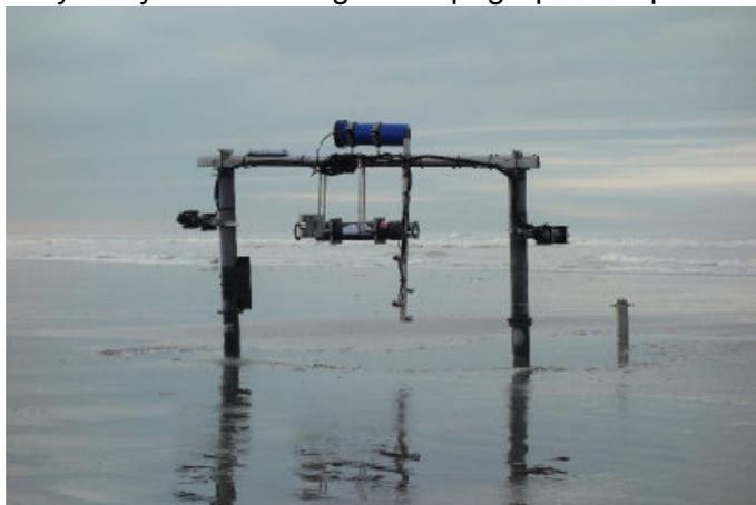
Figure 1 Measuring frame on the intertidal beach with equipment to measure wave height, flow velocity, suspended sediment concentrations, and grain size.
