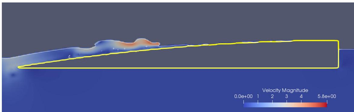
Figure 1 COMFLOW simulation of waves breaking over a parabolic floating reef.
