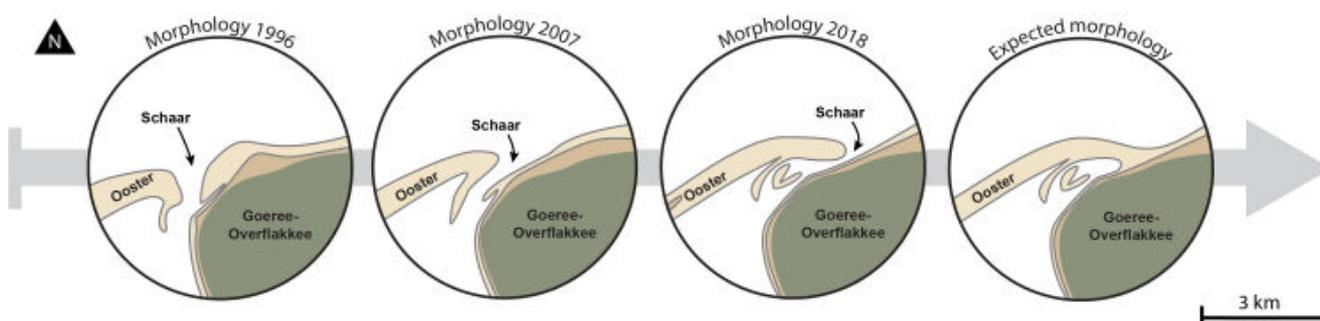
Figure 1 Schematization of morphological evolution of the Bollen van de Ooster near Goeree-Overflakkee and the expected future morphological development.
