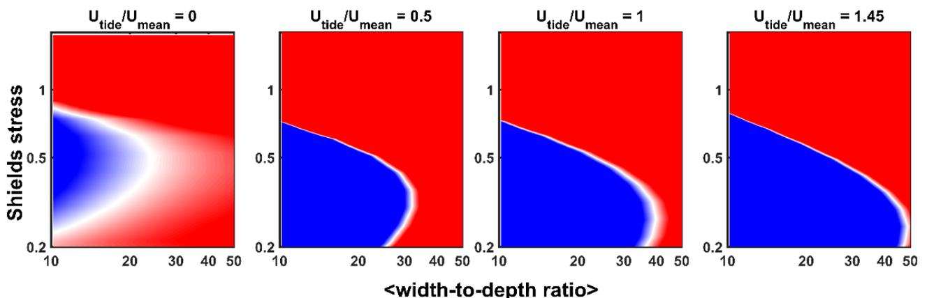
Figure 1 Stability of bifurcations for fluvial influenced ( $U_{\text{tide}}/U_0$  at the bifurcation = 0) and fluvial-tidal influenced cases with channel slope =  $3e-5$ . Red and blue indicates unstable and stable condition, respectively.  $U_{\text{tide}}$  and  $U_{\text{mean}}$  are tide-induced and tidally averaged flow magnitudes at the junction, respectively.
