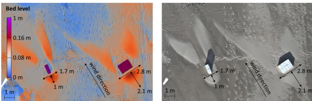
Figure 1 A DEM (left) and orthophoto (right) of the deposition around two scale models that vary in width
