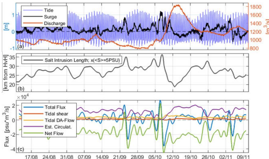
Figure 1 a) Forcing of the system; b) Salt intrusion into the system; c) Total tide-averaged salt flux (positive is inward) and contributions of the individual salt flux components, for location Maassluis (Rotterdam Waterway).
