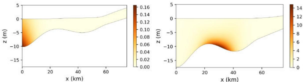
Figure 1 Modelled tidally averaged suspended sediment concentrations in ( $\text{kg}/\text{m}^3$ ) along the Loire estuary ( $x=0$  is the mouth) for bottom profiles representing the bathymetries around the years 1900 (a) and 2010 (b). The drastic increase in sediment concentrations is found by only increasing the depth, keeping all other model parameters constant.
