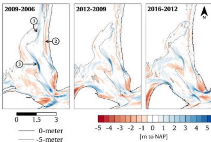
Figure 1 Bathymetric difference maps highlighting three main erosion/accretion characteristics. Isobaths based on 2009, 2012 and 2016 surveys, respectively.
