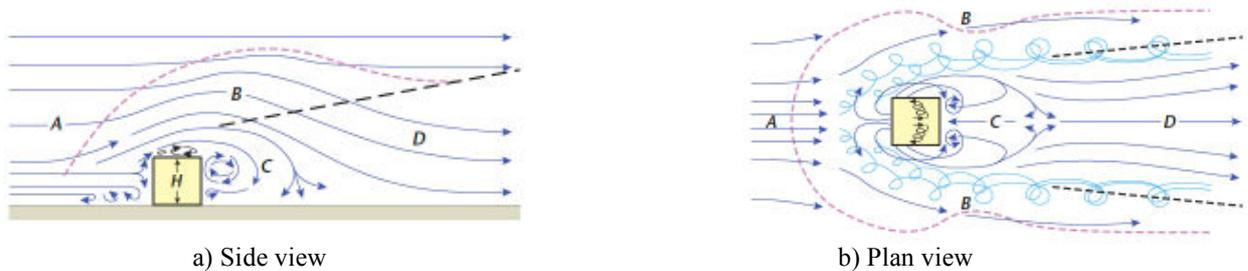
Figure 1 Airflow around an isolated cubic building a) side view, and b) plan view near ground level. A, B, C and D show the incident wind direction, displacement zone, cavity and the wake, respectively. [Oke et al., 2017]
