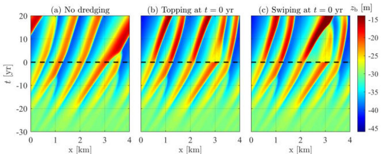
Figure 1 dredging the highest crest in a quasi-equilibrium sand wave field: (a) the undisturbed sand wave field (b) the topping of the highest sand wave crest and (c) swiping the topped sand volume to the trough to the left. This figure is adapted after Campmans et al. (subm.).
