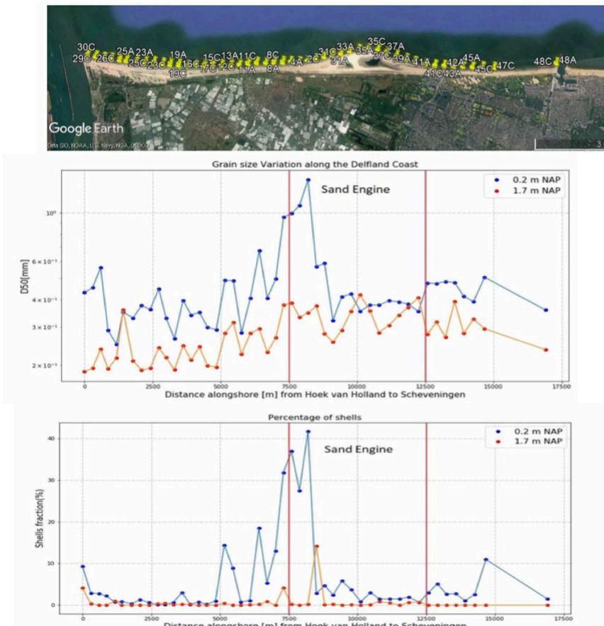
Figure 1 Spatial patterns in bed material along the Delfland coast. (Top) Sampling locations, (middle) median grain size at different levels, (bottom) shell fraction percentage. Source top panel: Google Earth.
