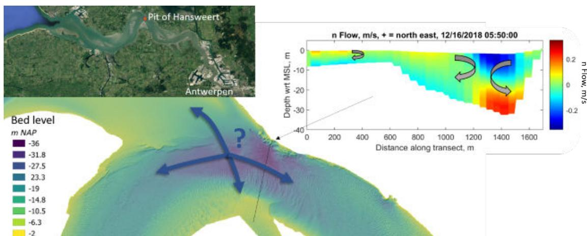
Figure 1 Bed level around the Pit of Hansweert, a pilot location in which 3 Mm<sup>3</sup> sediment is disposed for testing a new disposal strategy. Inset 1: overview Western Scheldt (Source: Google Earth). Inset 2: flow in n-direction.
