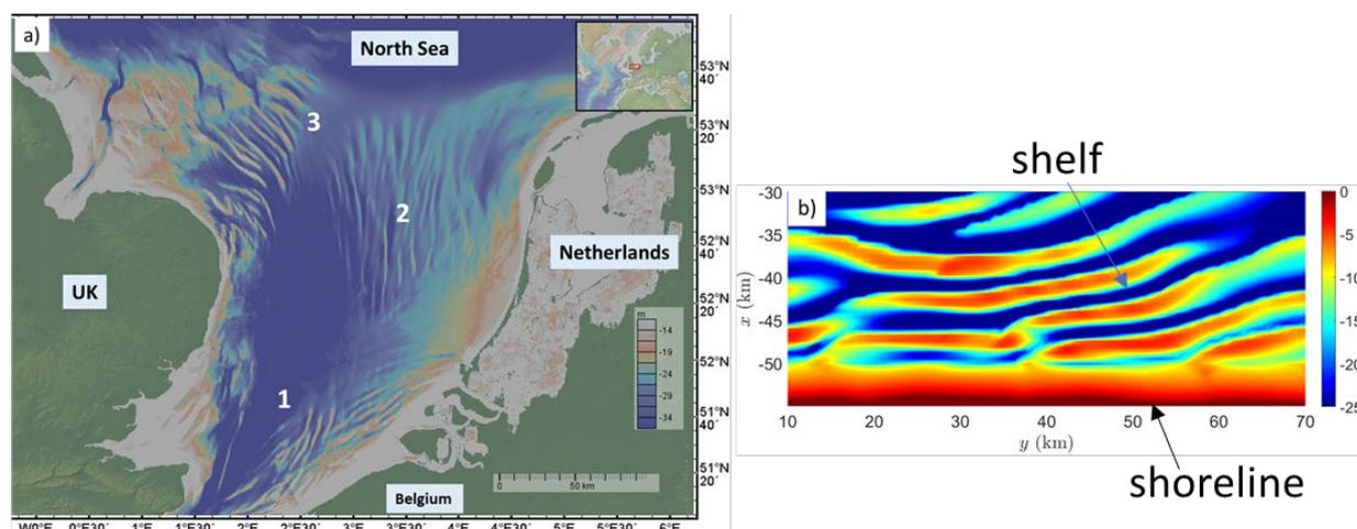
Figure 1 a) Bathymetric map of observed fields of tidal sand ridges (1, 2 and 3) in the North Sea. b) Simulated bed level after 500 years of morphodynamic evolution.
