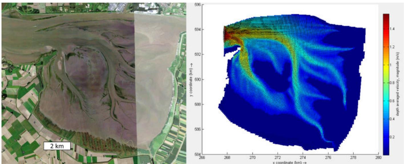
Figure 1 [left] Aerial photography of the Dollard basin along the Ems-Dollard estuary (source: google earth). [right] Example of model output with peak ebb flow velocities.
