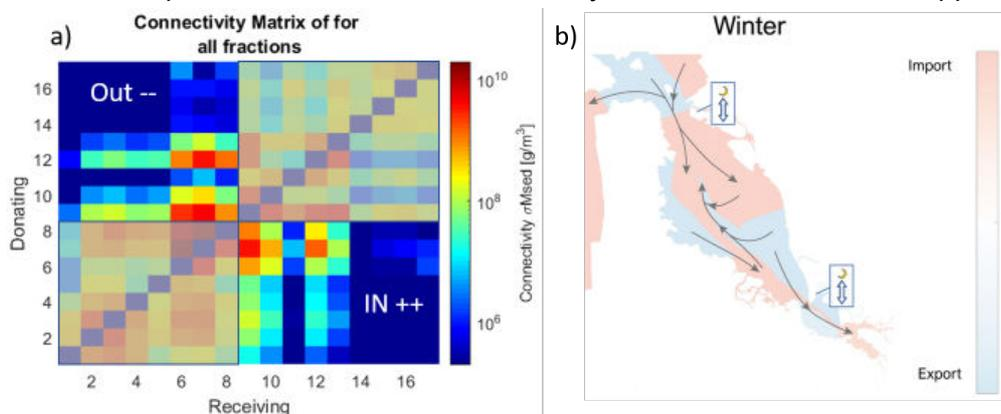
Figure 1 a) Connectivity Matrix for SFB in Spring indicating the incoming fluxes and outgoing fluxes with respect to South Bay during Winter (dec-feb). Each row represents outgoing fluxes from a certain segment and each column incoming fluxes. b) Concept Diagram with a schematization of the sediment fluxes, regions of import and export in Winter, with the tide being dominant in the sediment exchange at the South Bay entrance.
