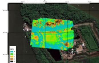
Figure 2 Example of georeferenced DEM overlay to satellite image.
