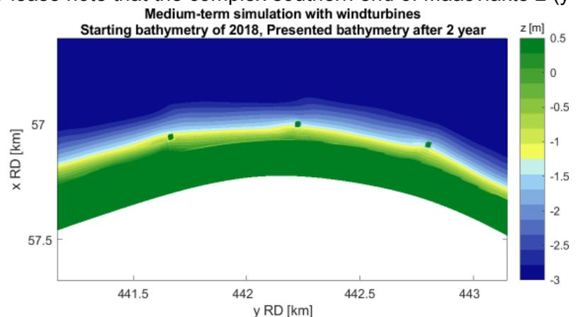
Figure 2 Simulation with wind turbines, final bed lay out.
