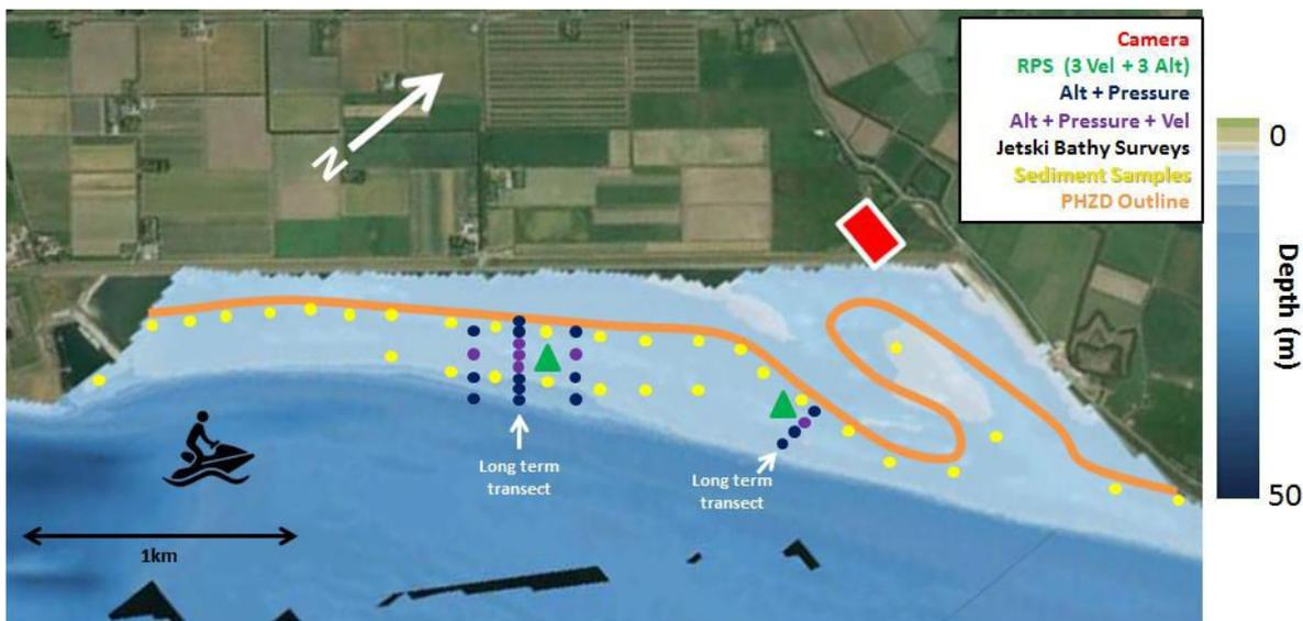
Figure 1 Schematic of planned field observations, including arrays of hydrodynamic sensors for short (monthly) and long (yearly) deployment (dark blue for pressure and depth, purple for pressure, depth, and velocity), a ripple scanner mounted on a frame with pressure and velocity sensors to capture bathymetric change (dark green). The orange line denotes the location of the seaward extent of the Prins Hendrikzanddijk.
