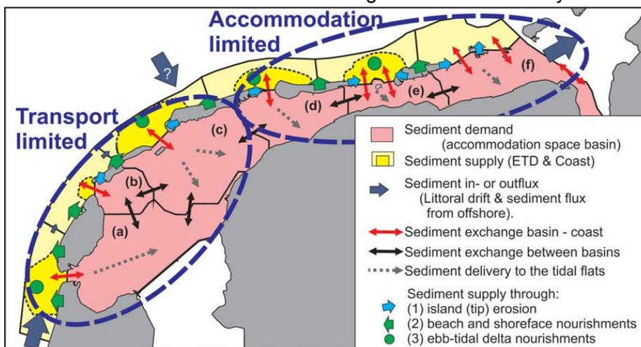
Figure 1 Schematic overview of transport limited and accommodation limited parts of the Wadden Sea (Wang et al., 2018)
