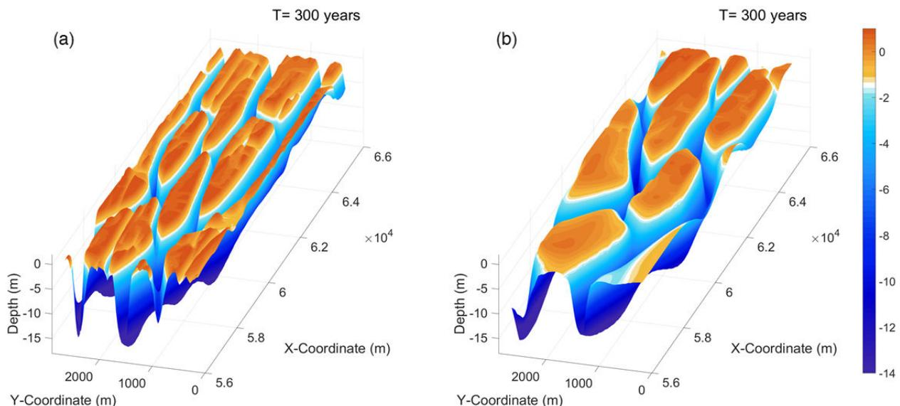
Figure 1 The modelled bathymetry (a) Flow only, and (b) Flow and Waves after 300 years for a section of the model domain. The white band represents the border between intertidal and subtidal areas.
