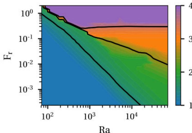
Figure 1 The four regimes (indicated by colours) dominated by transport due to (1) dispersion, (2) gravitational circulation, (3) momentum advection at a distinctive salinity front, (4) advection in a salt wedge. The regimes are plotted in the parameter space of the fresh water Froude number ( $Fr$ ; indicating discharge) and the estuarine Rayleigh number ( $Ra$ ; indicating mixing).
