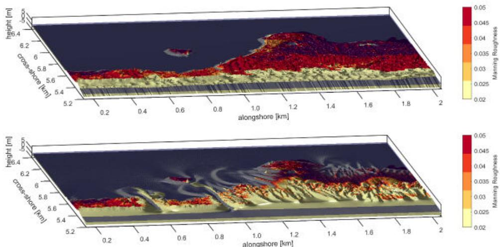
Figure 1 Pre- (top) and modeled post- (bottom) storm barrier island topography for Wilderness Breach – Fire Island (NY-USA) for hurricane Sandy. Color indicates bottom roughness as Manning values. MHW-level in blue for reference.
