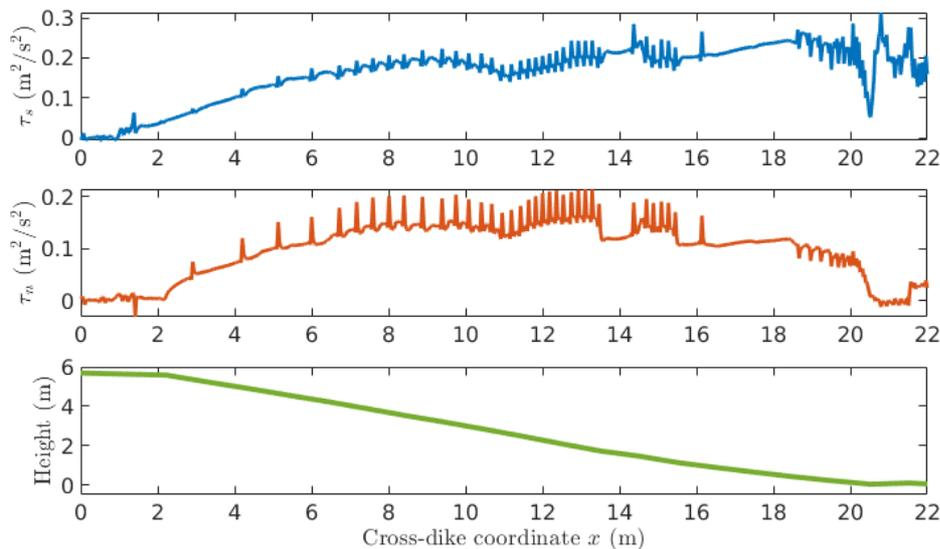
Figure 1 The shear stress  $\tau_s$  and normal stress  $\tau_n$  along the dike profile after 5 seconds of overtopping for an overtopping volume of 2500 l.
