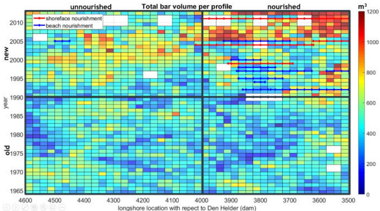
Figure 1 Timestacks of total bar volume (colors indicate  $m^3$ /longshore m) per transect (x-axis; left-right corresponds to south-north) between the years (y-axis; from bottom to top).
