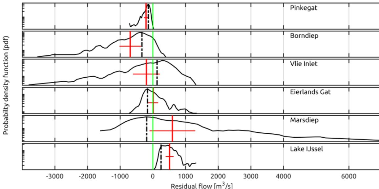
Figure 1 Probability density functions of monthly residual flows through selected tidal inlets. Positive flow indicates a transport into the Wadden Sea. The vertical red line marks the mean value; the black dashed-dotted line the median. The horizontal red line indicates the standard deviation. The analysis is done for the period 1979-2018.
