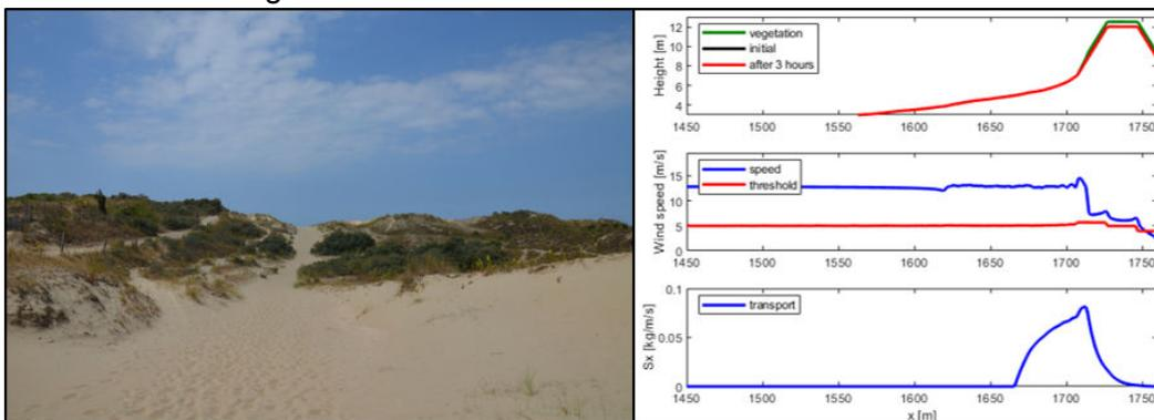
Figure 1 (left) Dune area at De Panne in the west of the Belgian coast. (right) Model simulation for a 3h wind event, with profile (top), wind speed (middle), and aeolian sand transport (bottom).
