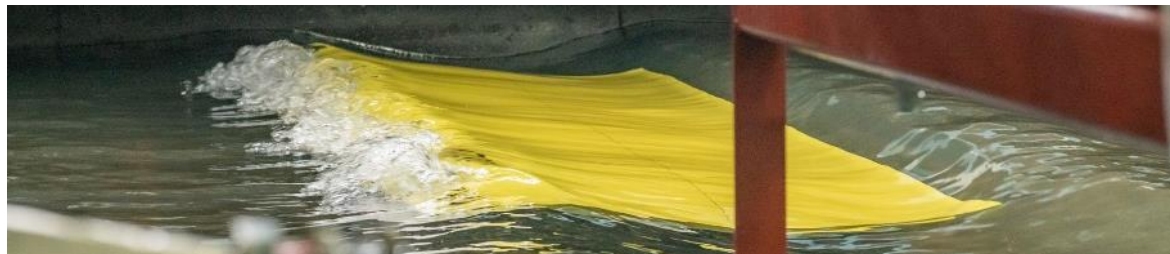
Figure: Waves breaking over the new floating breakwater design during scale model tests.
