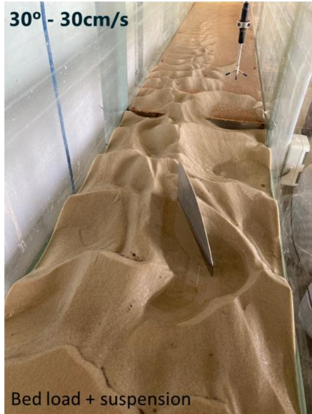
Figure 1: Flume experiments of the Sand Wing with mobile sand bed. Left: Sand Wing with 30° orientation; Right: no Sand Wing. Both experiments were performed with 0.3 m/s flow velocity.
