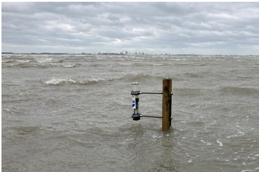
Figure 1: Monitoring short-term sediment dynamics with an acoustic SED-sensor during storm conditions in the Westerschelde (image courtesy: T. Grandjean).
