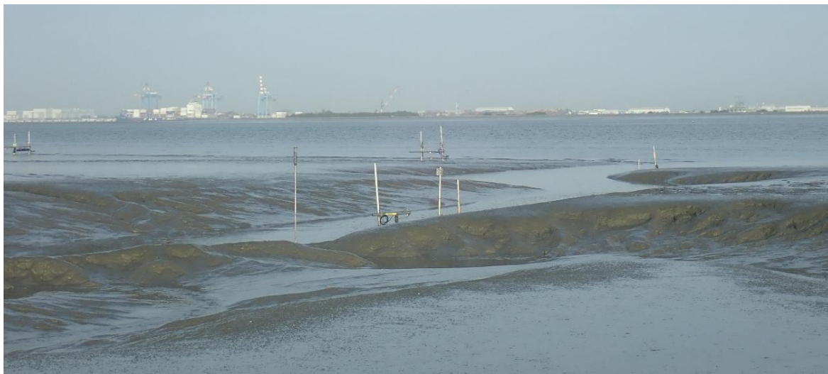
Figure 1: Frames with instruments placed in a creek and on the adjacent tidal flat in the Loire estuary.
