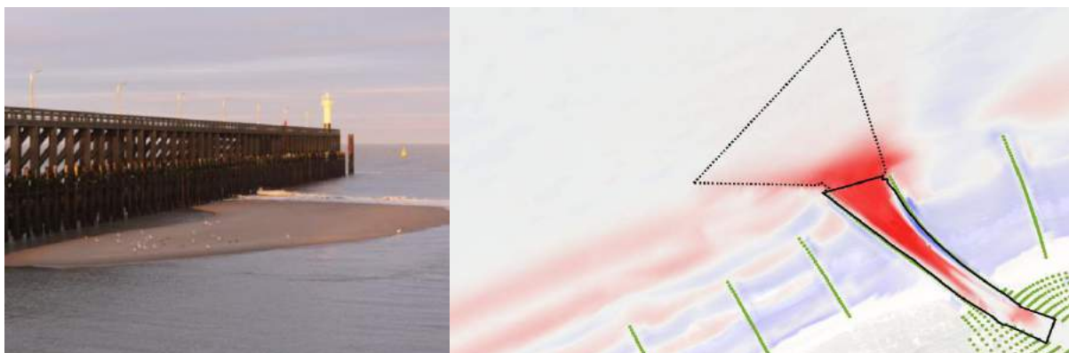
Figure 1. Illustration of the Blankenberge marina inlet sedimentation and XBeach model result of present situation.
