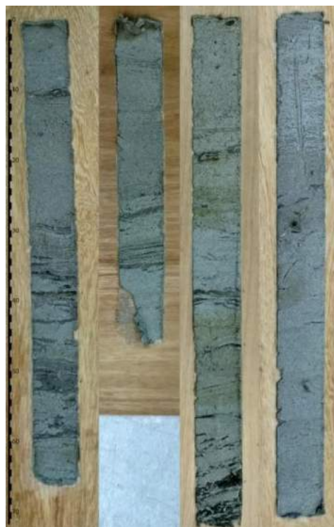
Figure 1. Lacquer peels of four sediment cores. Darker layers are mud layers.
