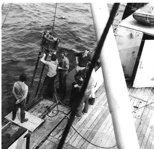
Figure 1. Sampling with a “Zenkovitch” vibrocorer in the late sixties.
