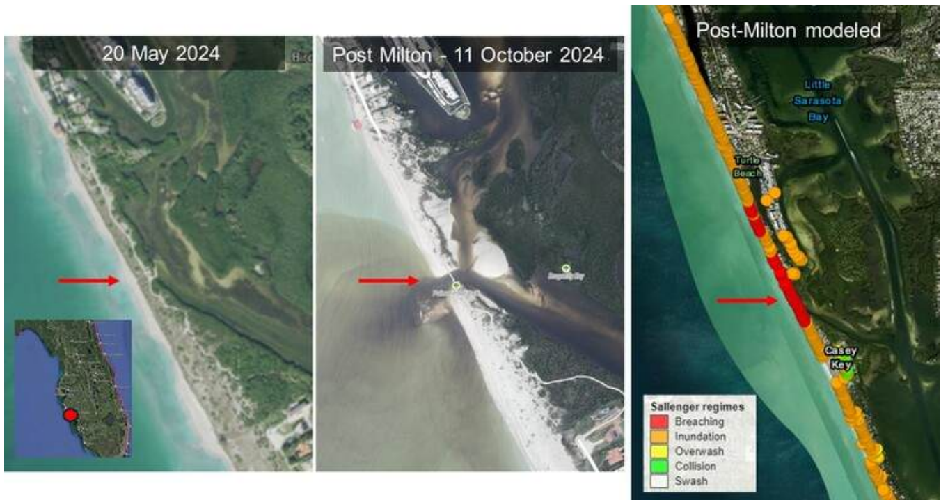
Figure 1: Pre-Helene/Milton imagery (left) and Post-Milton imagery (mid, source: NOAA) showing a small shallow breach and overwash deposits at Midnight Pass. The Xbeach model predicted breaching (right).
