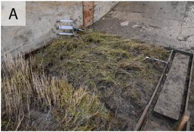
State of the saltmarsh at the toe of the dike after ca. 20 hours of wave exposure with the ADV deployed at the right side of the block (panel A) and maximum near-bed velocities for different states of the vegetation (panel B)
